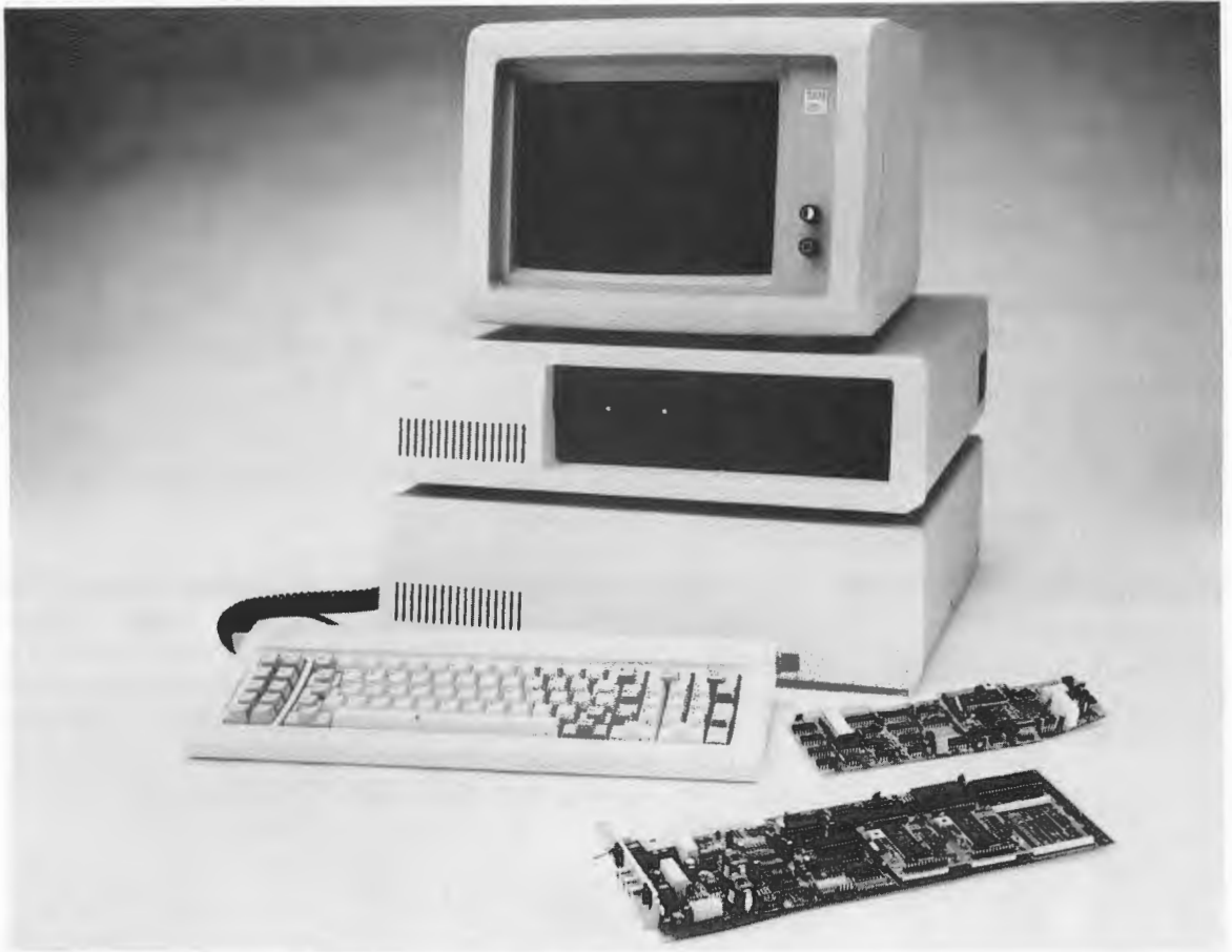
Fig. A-5. Tone dialing and decoding with the V100 voice synthesizer and Apple II or IBM computer (courtesy Vynet Corporation).
