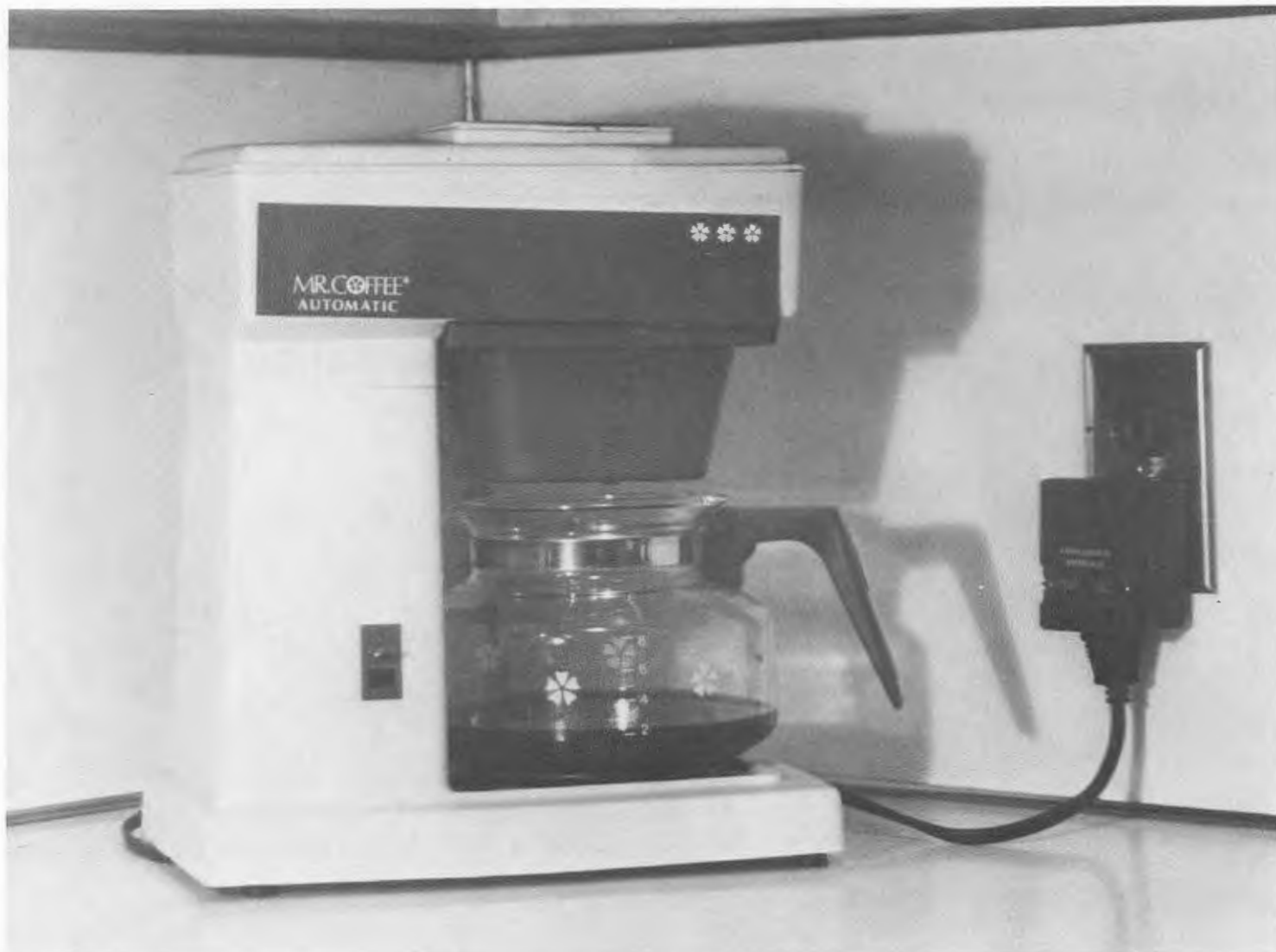
Fig. 18-15. The coffee is turned on from the master bedroom's X-10 Controller. The Home Control system checks to make sure it's turned off at the appropriate time.
