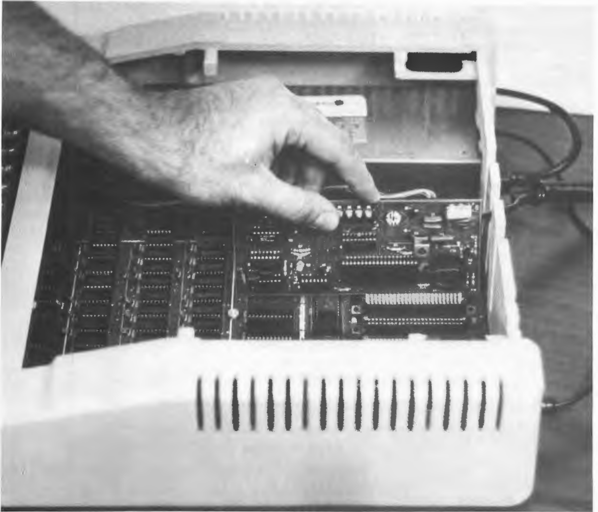
Fig. A-2. The EYE being inserted into an Apple II computer (courtesy Lehigh Valley Computer Corporation).
