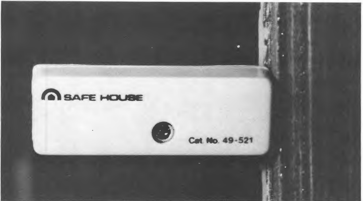
Fig. 18-18. A vibration window sensor monitors for unexpected guests in the den.
