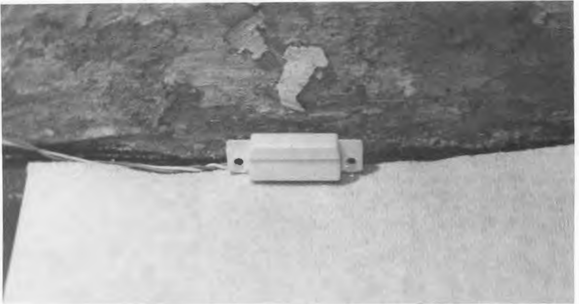
Fig. 18-23. If the basement floor becomes flooded, this moisture sensor will detect the condition. Note the paper towel used to absorb water and speed detection.
